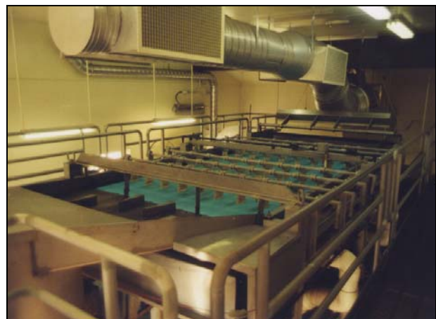
Gravity belt thickener.
